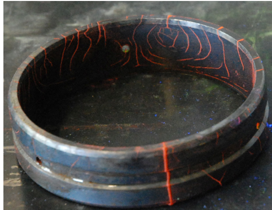
Crack indication resulted from application of the water-based suspension prepared by use of MEF 515 dry concentrate.
