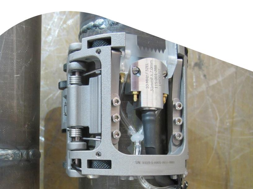
NDT inspections of circumferential butt welds are a complex task. This type of joint is found in various structures including small diameter tubes in boilers. Experts inspect these to find defects which could result in the failure of a component, possibly inducing a human or environmental hazard.
